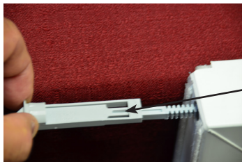
4. Tilt Latch inserted into Cup from left
